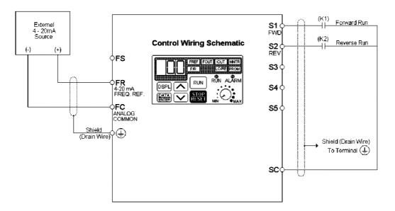
This configuration is used when the start & stop signals and the frequency reference come from a remote source, such as a PLC. It can also be used with a maintained switch when it is desirable to have the Drive restart on restoration of power. It should not be used where safety of attending personnel might be threatened by a restart.
