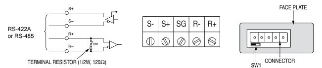
Cable must be assembled per pin-out diagram shown below.
