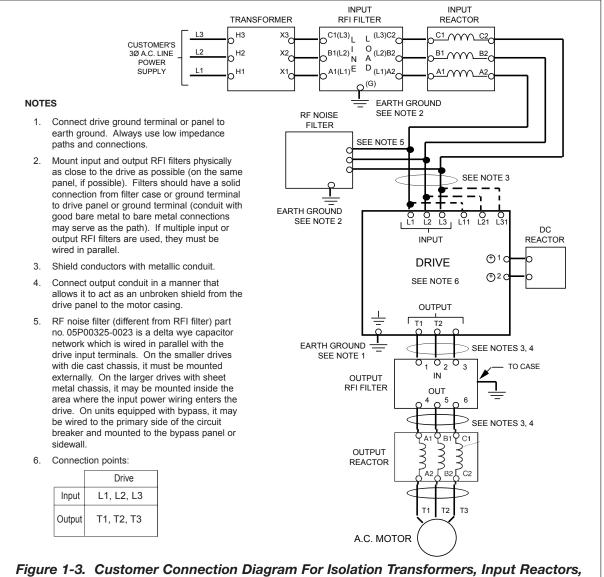
Input RFI Filters, DC Reactors, Output Reactors and Output RFI Filters
