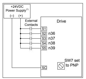
External wiring for PNP inputs
