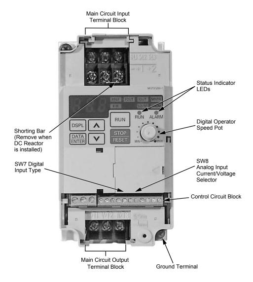
Figure 1-1. Component Identification (Sheet 1 of 2)
