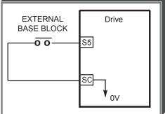
When both the Forward Run command and Reverse Run command are open, and the external Base Block command is applied (i.e. contact closed), coast stop is accomplished and after a 20 msec delay the frequency command is changed to 0Hz. When the Base Block command is removed, the Drive will remain in stopped condition until Forward Run command or Reverse Run command is again applied.
