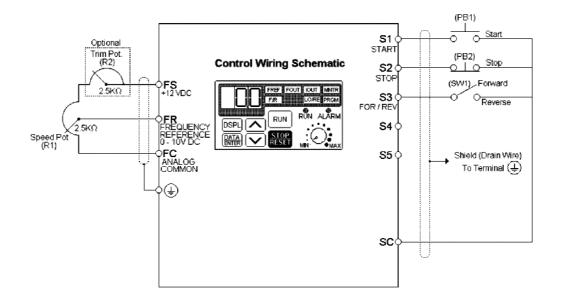
This configuration is best when a person rather than an external controller (PLC, relay, etc.) controls the Drive. Both potentiometers ((R1) & (R2)) should have a resistance value between  $2000\Omega$  and  $3000\Omega$  and be rated for at least 1 Watt. The trim pot is optional, but without it the manual speed pot will output 10V (60 Hz) at just three-quarters of its rotation.
