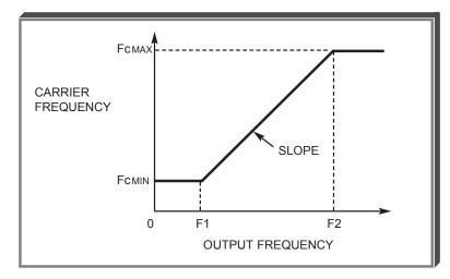
Carrier frequency should be decreased as the distance between the Drive and the motor increases, to reduce capacitive coupling in the motor leads.
