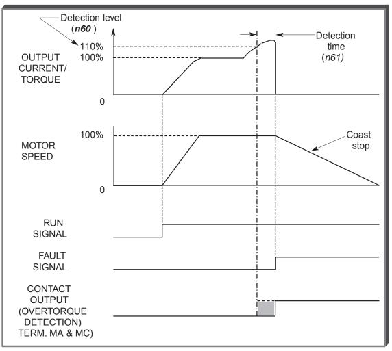
**Overtorque Detection Timing Diagram**
