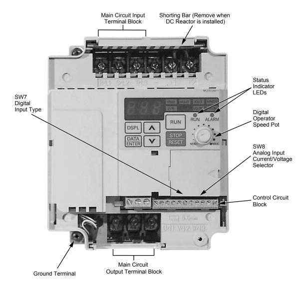
Figure 1-1. Component Identification (Sheet 2 of 2)
